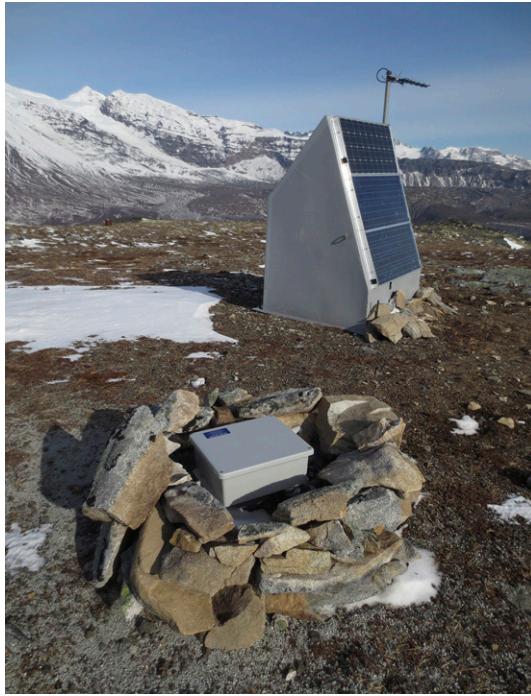
A continent-wide network of seismometers like this one, which was installed in south-central Alaska in 2016, helps researchers probe Earth's inner structure. Image credit: EarthScope National Office , a National Science Foundation funded project/Max Kaufman. EarthScope scientists study the structure and evolution of the North American continent using three primary observatories, the Plate Boundary Observatory, US Array, and the San Andreas Observatory at Depth. For more information, visit www.earthscope.org .
